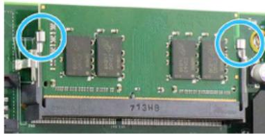
3. Gently pull on the memory module to remove it from the board.
