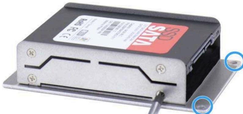
5. Connect the previously disconnected cable to the installed SSD and gently put the tray back into the system with the connector side being inserted into the system first and secure the tray with three screws.
