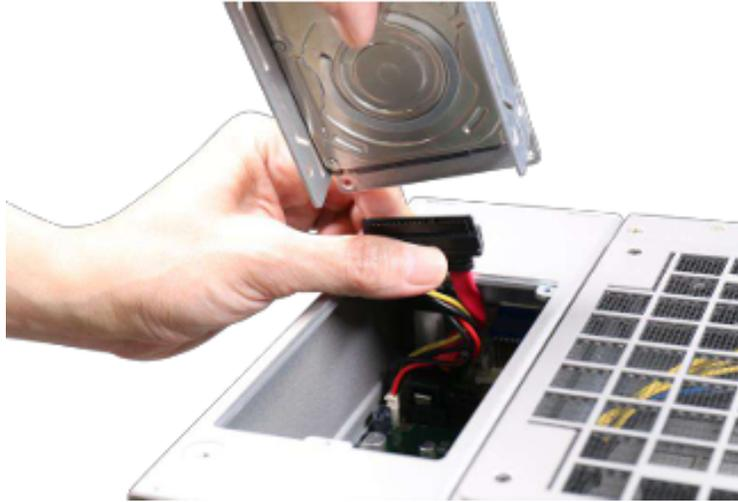
3. Place the SSD (with labels facing up) and unscrew the four screws on the side of the tray. Take out the old SSD and safely discard it.
